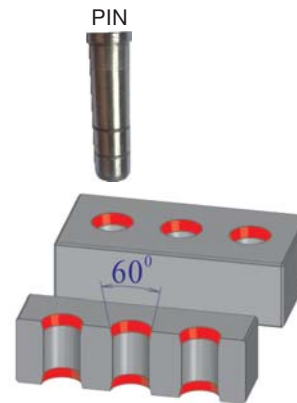
Chamfer with 60^\circ used for deburring before "pin". 60^\circ chamfer is easier than 90^\circ or 120^\circ to locate the pin.
