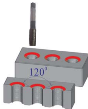
Chamfer with 120^\circ used for tap holes, which reduce the loss of threads.
