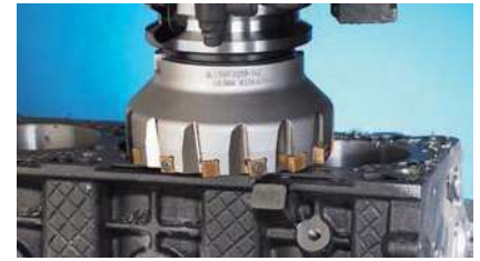
Roughing for cast iron
