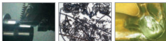
Conventional chip breaker
