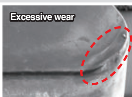
Existing grade (K10)
