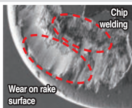
Existing grade (K15)
