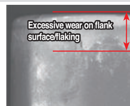
Existing grade (K15)
