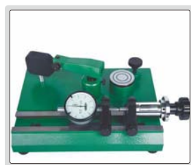
inspect accuracy of dial indicators (range 0-25mm)
