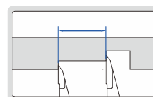
jaws with different height used for measuring the distance in different level
