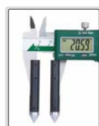
measuring center distance
