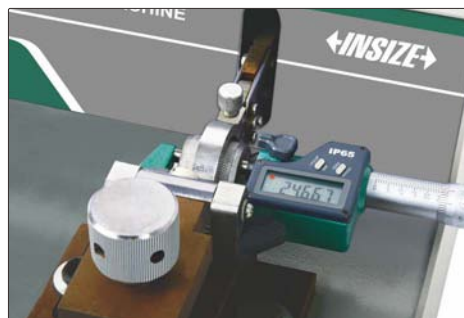
lapping measuring surfaces of outside micrometer
