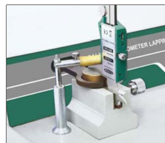
lapping measuring surfaces of caliper lower jaws
