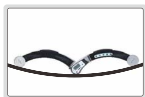
internal diameter measurement
