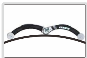
external diameter measurement
