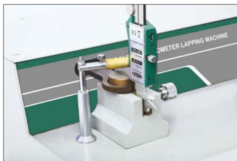
lapping measuring surfaces of caliper lower jaws
