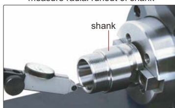
measure radial runout of shank
