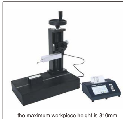
heavy duty test stand (optional)
