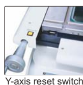
Y-axis reset switch
